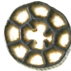
Attached Growth on MBBR and IFAS Media Surface
