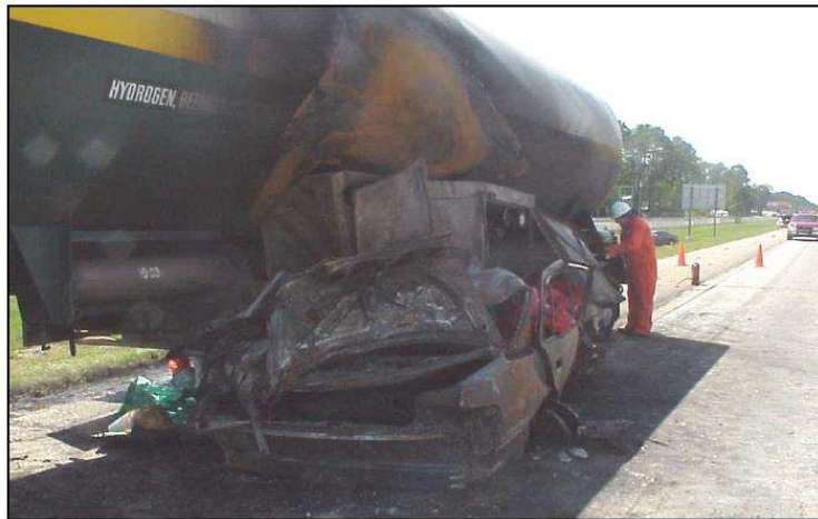
The car and hydrogen trailer after the fire was extinguished
